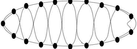
Figure 23.3: Two edge-disjoint Hamiltonian paths spanning a set of nodes.
