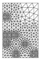
Figure 19.1: A well-shaped triangulation
