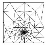
Figure 12.1: Triangulation of well-spaced point set around a singularity
