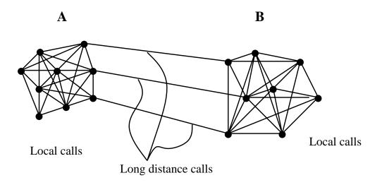
Figure 17.2: Partitioning of a telephone net as an example for a graph comparable in cost
