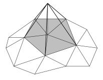
Figure 12.3: A basis function for 2D finite element
