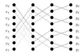
Figure 10.3: FFT network for 8 elements. (Such a network is not built in practice)
