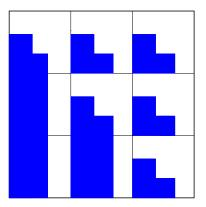
Figure 13.5: A stage in Gaussian elimination using cyclic order, where the shaded portion refers to the zeros and the unshaded refers to the non-zero elements
