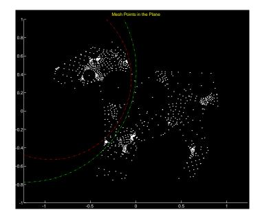
Figure 17.13: This partitions the mesh into two pieces with about n/2 points each, connected by at most O(sqrt(n)) edges. These connecting edges are called an "edge separator".
