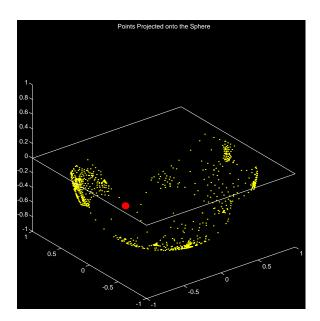
Figure 17.8: First we project the points stereographically from the plane onto a sphere (of one higher dimension than the mesh); Now we compute a "centerpoint" for the projected points in 3-space. Every plane through the centerpoint separates the input points into two roughly equal subsets. (Actually it's too expensive to compute a real centerpoint, so we use a fast, randomized heuristic to find a pretty good approximation.
