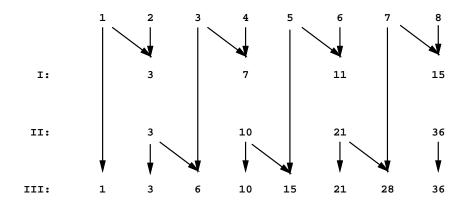
Figure 10.1: Action of the Parallel Prefix algorithm. The array in II comes from running scan recursively on the array in I.
