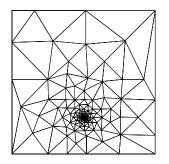
Figure 18.2: Triangulation of well-spaced point set around a singularity
