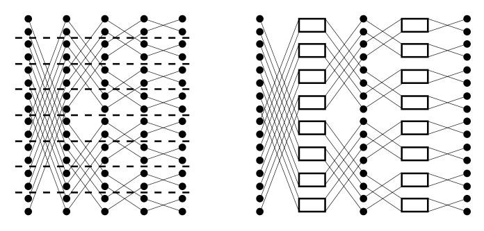
Figure 10.5: Left: more than one element per processor. Right: one box is a  $4 \times 4$  matrix multiply.
