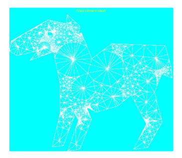
Figure 17.6: The input is a mesh with specified coordinates. Every triangle must be "well-shaped", which means that no angle can be too small. **Remarks:** The mesh is a subgraph of the intersection graph of a set of disks, one centered at each mesh point. Because the triangles are well-shaped, only a bounded number of disks can overlap any point, and the mesh is an "alpha-overlap graph". This implies that it has a good separator, which we proceed to find.
