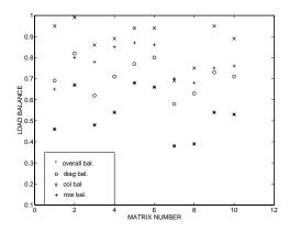
Figure 14.5: Efficiency bounds for 2-D cyclic mapping due to row, column and diagonal imbalances (P = 64, B = 48).
