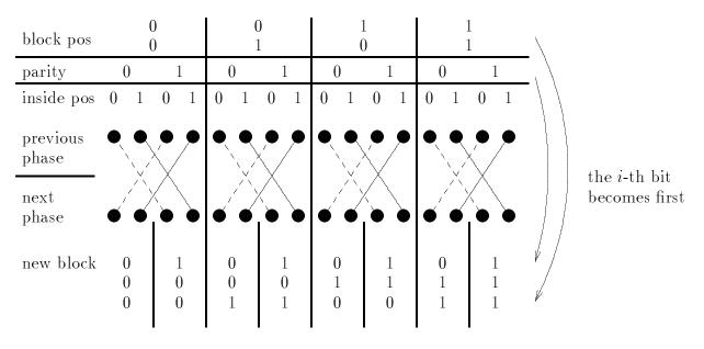
Figure 10.4: The output of FFT is in bit-reversed order.
