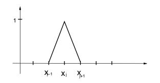
Figure 12.2: A basis function for 1D finite element
