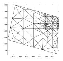
Figure 18.4: A well-shaped mesh generated by quad-tree refinement
