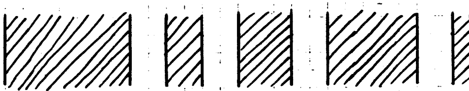
Figure III.14: The experimental cumulative distribution function for five wires of widths 7,2,3,5,1. The spacing required between wires is 2 units, thus l_2 = 9 , l_3 = 13 , etc.
