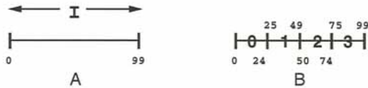
Figure 2-2: Partitioning a 100-iteration 1-D loop: (a) the iteration space, (b) the partitioned iteration space.
