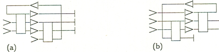
FIG. 7.1 (a) A conservative-logic network and (b) its inverse.
