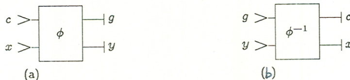
FIG. 7.2 (a) Computation of y = f(x) by means of a combinational conservative-logic network \phi . (b) This computation is “undone” by the inverse network, \phi^{-1} .
