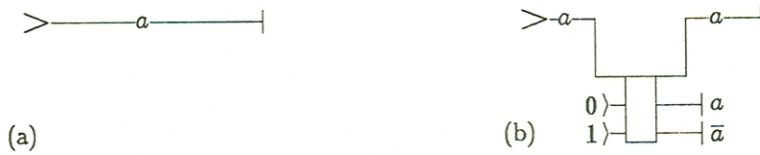
FIG. 7.4 The value a carried by an arbitrary line (a) can be inspected in a nondestructive way by the “spy” device in (b).
